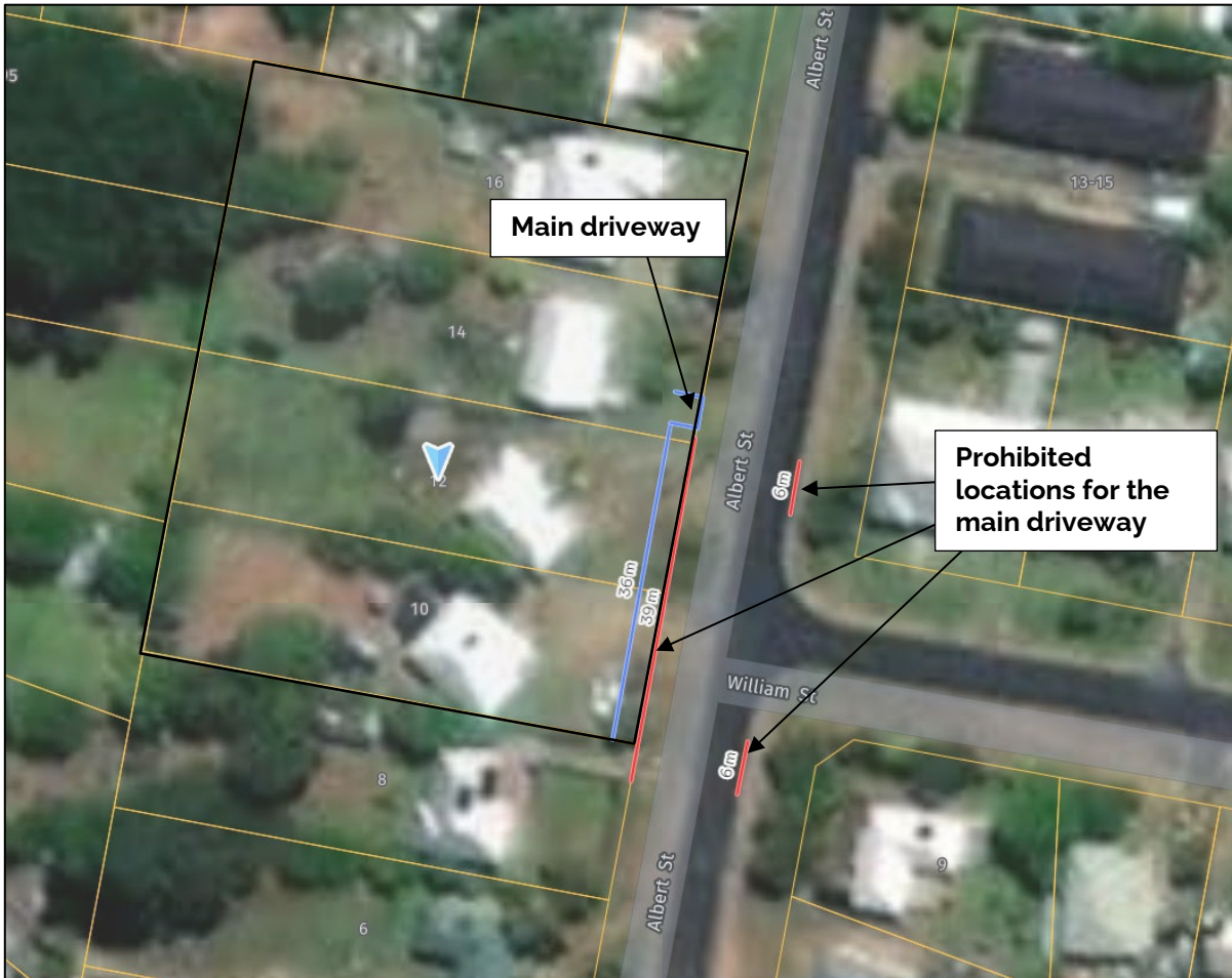
Figure 9: Location of the main driveway with respect to the prohibited locations of access driveways
